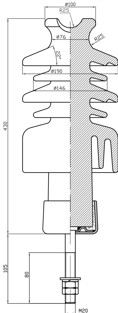
**SÚ ĐỠ ĐƯỜNG DÂY 35KV CHỐNG NHIỄM MẶN(P12.5 ET200L CD900)**
